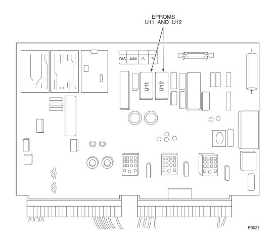
Figure 2-11. Main PCB (Model TC200) EPROM Replacement
